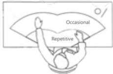
Centrally located user controls reduce instances of twisting and over-reaching.
